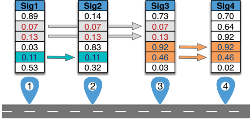
Figure 3: If \phi = 2/6 , the path [1, 2, 3] and [3, 4] are both \phi -consistent paths. We can estimate the cardinality of mobile entities visiting at least one checkpoint on path [1, 2, 3] as (6 - 1)/(0.14 + 0.07 + 0.13 + 0.03 + 0.11 + 0.03) \approx 10 . Multiplied by the Jaccard similarity of the path, 2/6 , the number of mobile entities sharing the path is 3. Hence the path is a \psi -popular path if \psi = 3 .
