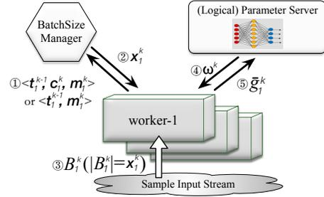
Fig. 5: LB-BSP workflow in iteration  $k$  (the circled numbers represent the execution order). The logical PS can be in the form of distributed shards, or be replaced by the All-Reduce architecture.
