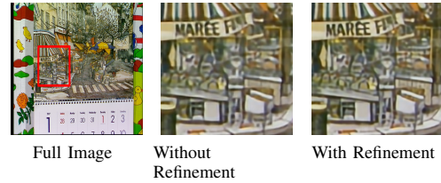
Fig. 6. Visual comparison of the effect of refinement with 3 frames input.
